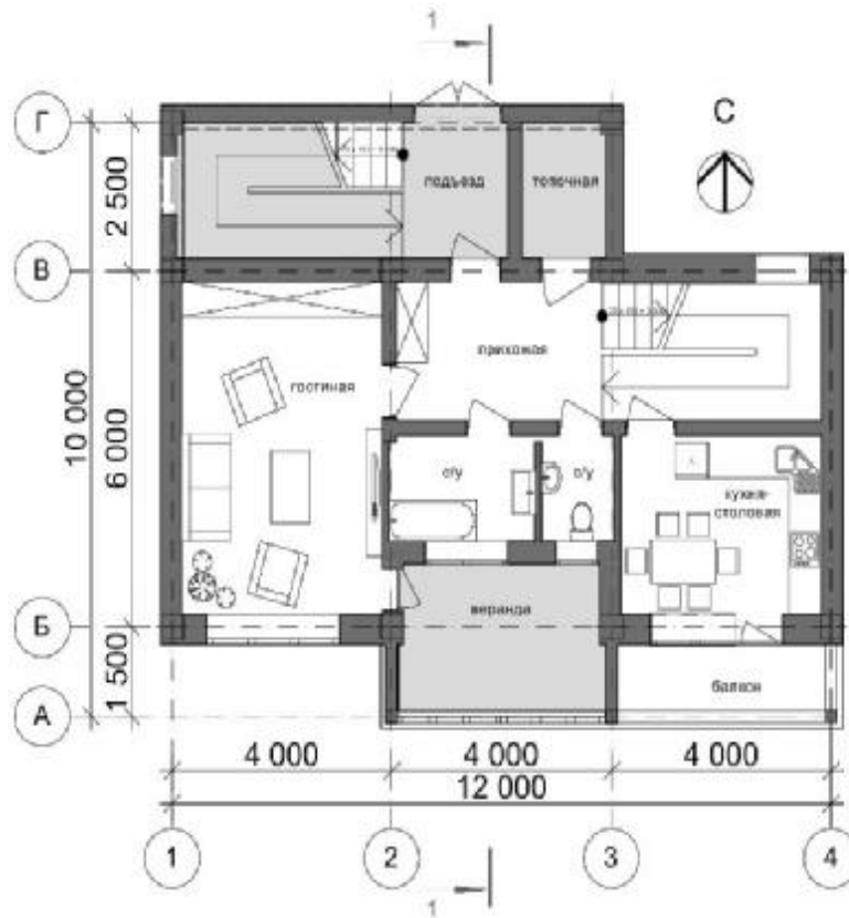
Fig. 1. Plan of the ground and the first floor of the flat in the energy-efficient 4-storey building with a block ability
