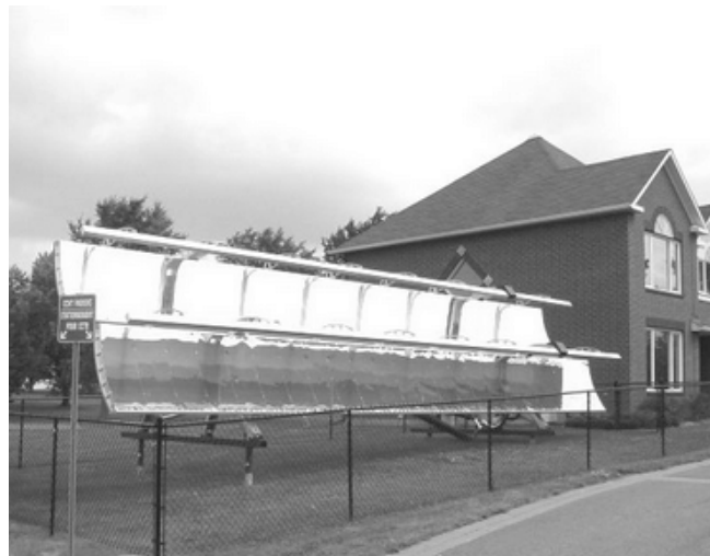
Fig. 3. Parabolic trough concentrator for the receipt of hot water
