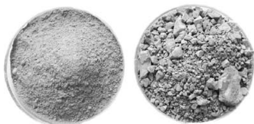
Fig. 1. Silica Fume images: SF-1 undensified form (left); SF-2 aggregated form (right)
